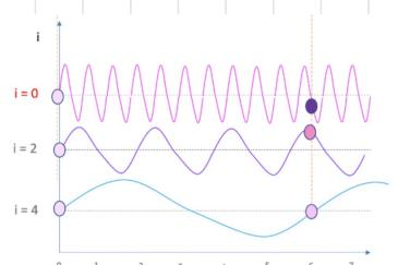
$$\begin{aligned} E_t &= \left[ \begin{array}{c} \vdots \\ e^{i0t} \\ e^{i1t} \\ \vdots \\ e^{i(n-1)t} \end{array} \right] \quad \theta = \frac{1}{10000^{2k/d}} \end{aligned}$$
